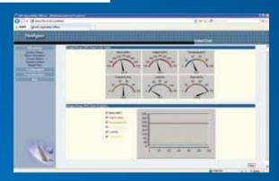
Software support most OS for remote monitor and control UPS through LAN, warning notifications through broadcast and
